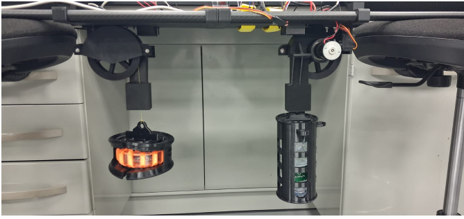
Fig. 6. Passive Two-Stage Rotary-Damper Design
